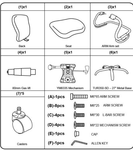
Insert and loosely tighten all screws. When assembly is completed, fully tighten all screws before using. This chair is only intended for sitting. Any other use will void the warranty.
